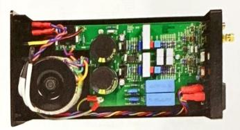
Inside the Pellar has a substantial on-board power supply.
